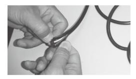
**Step 3:** Use a long nose plier to remove the jackets of the 3 wires.
