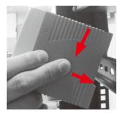
**Step 2:** Check whether the DIN rail is tightly on the track.
