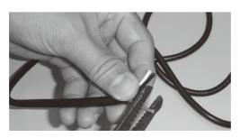
**Step 4:** Make sure the wires are neatly straightened.
