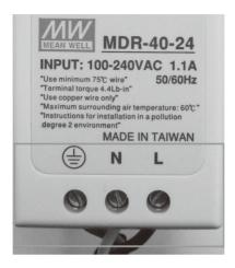
Figure 1: Connecting the 3 wires to the corresponding location
