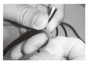
**Step 5:** The 3 wires should consist of a live wire, neutral wire and earth wire.
